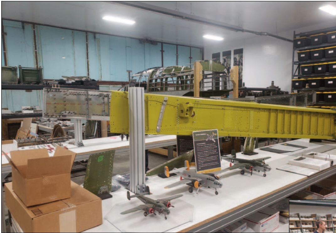
Left and below: The two wing spars, one restored, the other built from scratch/plans.
