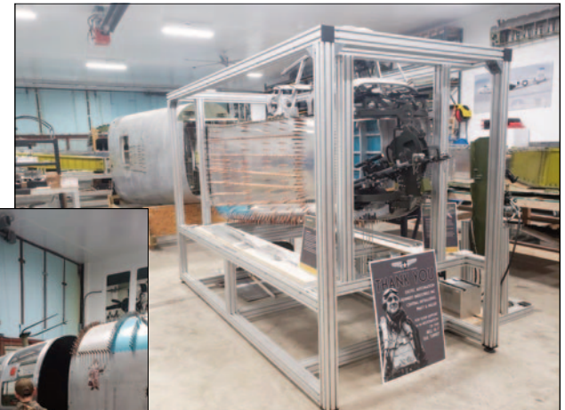
Above: Tail/rear fuselage gunner turret area is enclosed in cradle to facilitate transport for display and demonstration off-site. The gun movements work!
