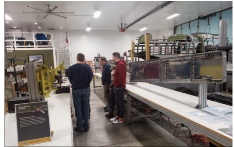
Left and below: The two wing spars, one restored, the other built from scratch/plans.
