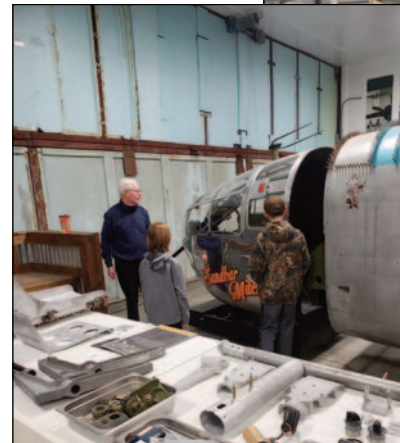
Above: Tail/rear fuselage gunner turret area is enclosed in cradle to facilitate transport for display and demonstration off-site. The gun movements work!
