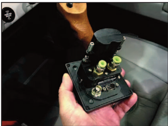
The uAvionix AV-30 has a built-in battery that's accessed from the rear chassis.
