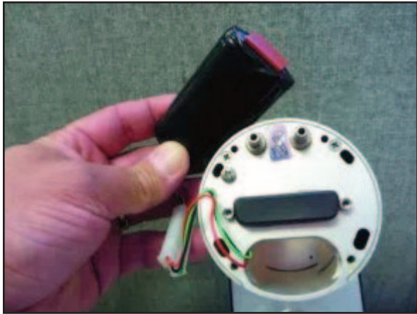
The four-hour rechargeable backup battery attached to the rear chassis on Garmin's G5 has a mandatory yearly inspection interval.
