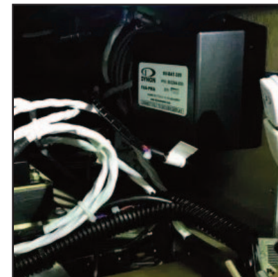
Dynon's SkyView HDX Certified big-screen EFIS has a remote battery installed behind the panel in a Cessna.
