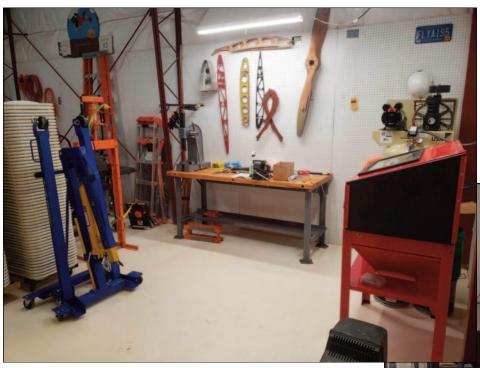
Above: Maintenance area off the main hangar bay, including a brand new grit blaster cabinet donated by Loren Duke. Jim Brown will have attached the air system to it by the time you read this. The hydraulic arbor press is affixed to the floor and ready for use. There's also a mechanical bench arbor and a vise, but we need more. You can never have enough vises, right?
