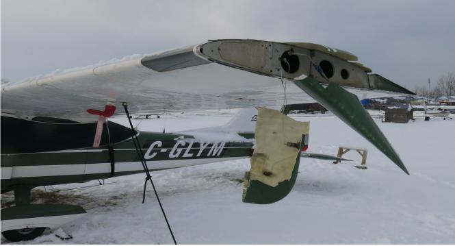
Figure 3: Damage to left wing
