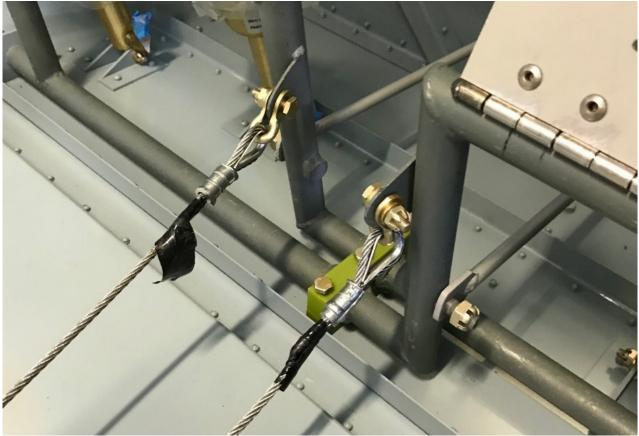
Figure 6: Rudder cables and shackles at the pedals.
