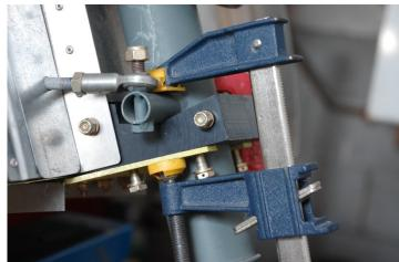
Figure 1: Nosewheel strut clamped to its' centre or neutral position at the bottom of the "V" notch in the strut bearing block.
