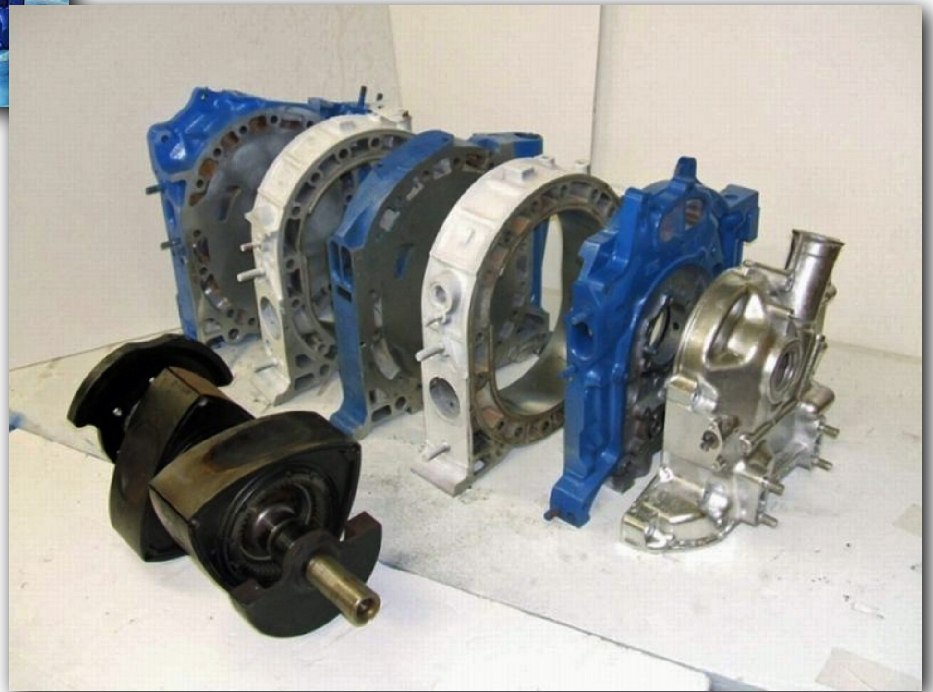
Photo 4: Exploded Block and Moving Parts
