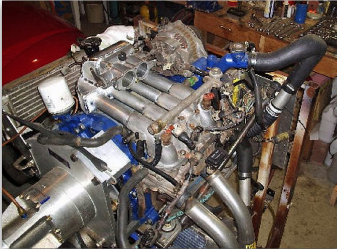
Photo 6: Custom Intake and Geared Drive
