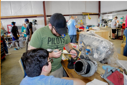
Alex showing Max the proper way to measure the inside diameter of a cylinder
