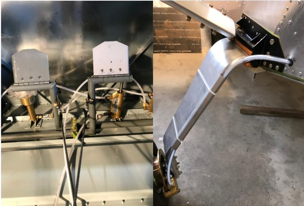
The Cruzler has dual brakes and brake lines were fitted using tubing specified by Matco for their brake assemblies. Brake lines were routed to exit the fuselage at the sides just behind the main gear attachment brackets and then follow trailing edges of the gear legs to each caliper. A metal protective shroud was temporarily secured with zip ties.
