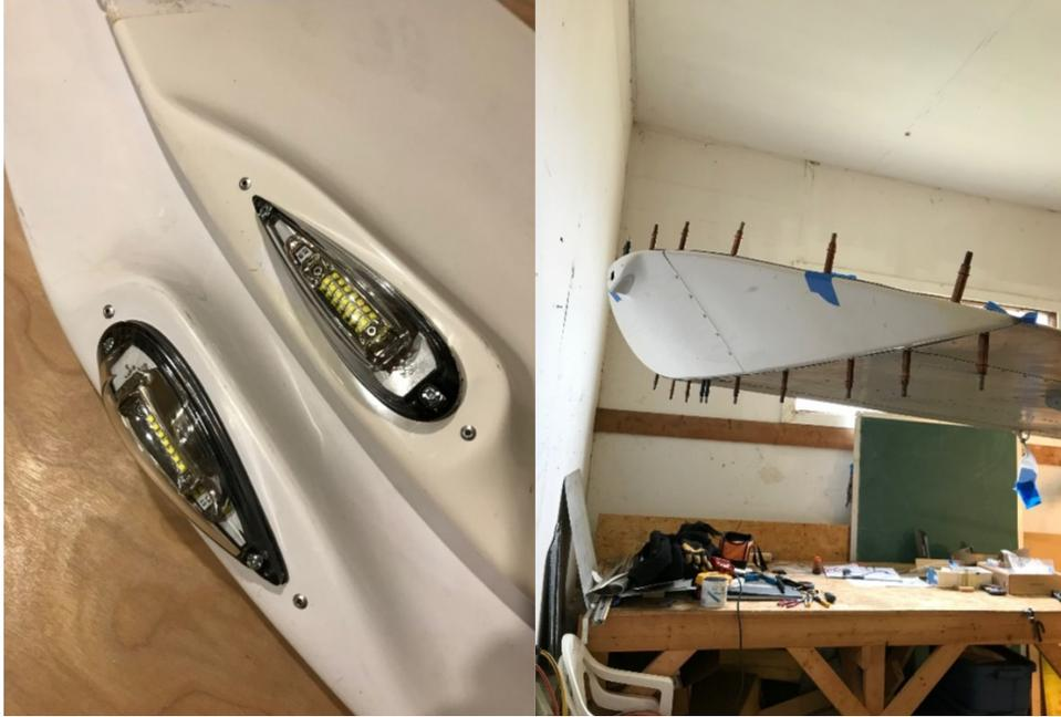
AVEO Engineering LED wingtip lights were acquired and fitted to the plastic wingtips. The wingtips were fitted to the wings and drilled ready for riveting. The lights were installed so that they can be removed as their own inspection panels to access wiring connections just inside the wingtips.
