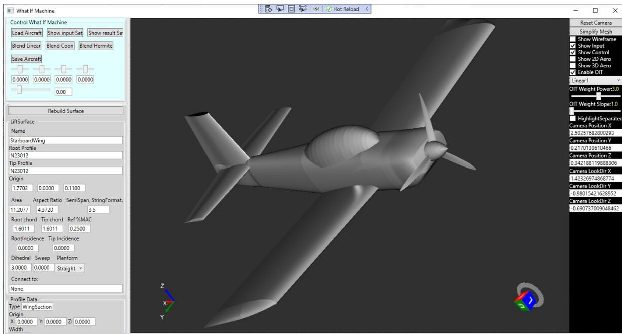
This is a model approximation of the RV8.. (The left pane shows the parameters used to define the starboard wing) If the Aspect ratio and planform are changed we get the next image : sort of an RV-Spitfire....
