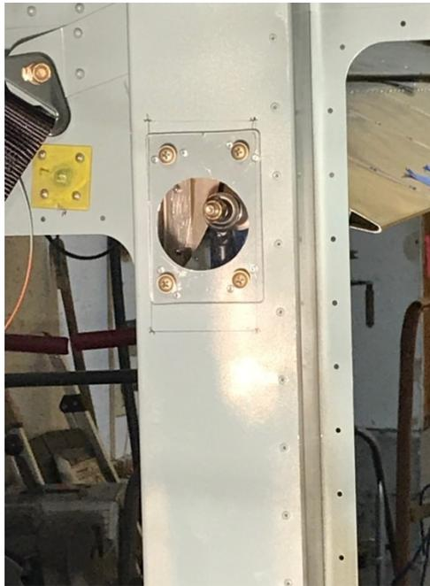
An access opening was made for each upper flaperon linkage which is required for installation of the control rods. Cover plates were fabricated from clear Lexan and installed with nut plates. The idea was to facilitate easy inspection of the linkages.
