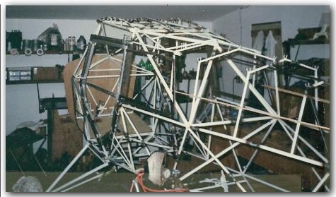
the lower structure that the boot cowling attaches to. First you have to fabricate and install both the instrument panel and firewall, then decipher the drawings for what to do with the 3/8" Piper channel. Trying to bend U-Channel to create curved sides that blend into a perfectly flat, level and square form is not initially obvious. In addition to seeing the big picture is the difficult practicality of welding 0.015" U-Channel onto main
