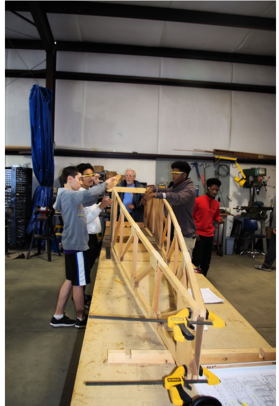
The sides of the 2 place Pietenpol being fixed into place and actually starting to take the shape of a fuselage.
