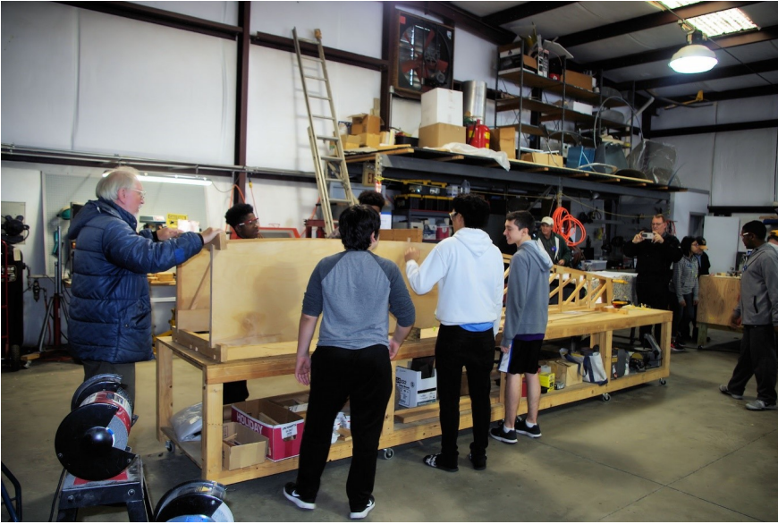
The sides of the 2 place Pietenpol being fixed into place and actually starting to take the shape of a fuselage.
