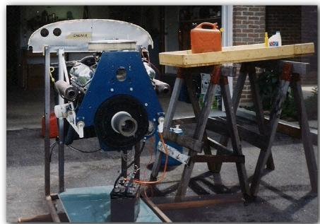
was well cranked over with no plugs to clear out those oil squirts. It huffed, smoked, fouled plugs and backfired at least once before it came to life. Within 10 seconds of operating there was glycol leaking all over the place, WTF!! Two of the front end frost plugs had corroded right through; of course they were behind the reduction
