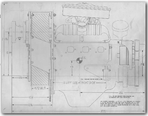
The drive itself is made from super charger blower sprockets (9.77" and 4.88"), three large bearings, some aluminum channel and backing plates. The front plate had to be machined for belt tightening groves, have a bearing bolted on to carry torsion loads from the crankshaft lower sprocket and a floating bearing block assembly that mated to the upper sprocket and adjustment grooves. The prop
