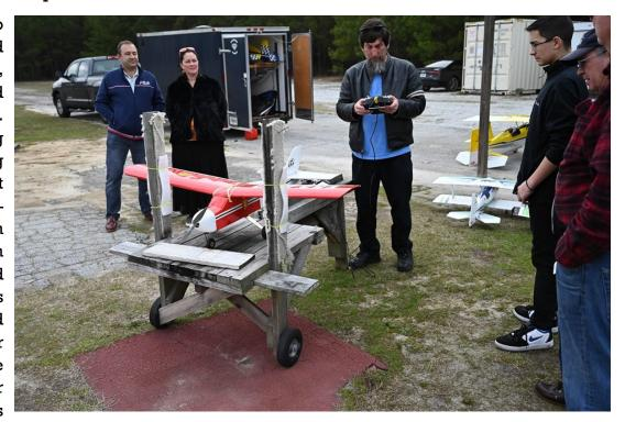
are available. Finally, they are covered with a mylar iron-on covering instead of cloth, though larger RC aircraft may use nearly identical (lighter weight) cloth to their larger cousins.
