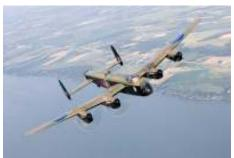
The Lancaster was the Allied Command's "Best of the Bombers". Powered by four Rolls Royce or Packard-built Merlin engines, it was the only aircraft capable of carrying the 22,000 pound "Grad-Slam" bomb. It had speed, ceiling, and lifting power that no other aircraft of the day could match. Weighing 36,000 lbs empty, it was capable of lifting another 33,100 pounds of fuel and bombs.
