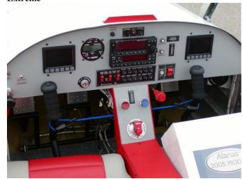
Photo 7 Instrument Panel for the Zodiac XL SLSA <a href="http://www.newplane.com/amd/amd/601">http://www.newplane.com/amd/amd/601</a> SLSA/601.html
