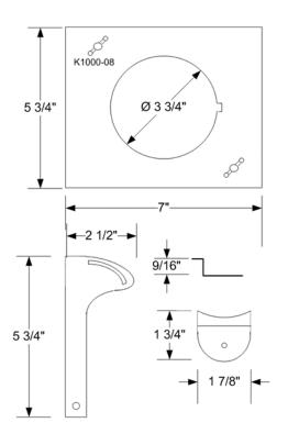
Once everything was primed, I riveted it together. The side angle pieces with the slot get riveted to the back of the plate using AN426AD3-3 rivets. The lamp clamps are held on with K1000-08 nutplates and AN515-898 screws.
