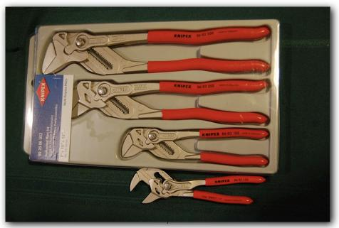
Figure 4 – Knipex 86-Series Plier Wrenches in 150mm, 180mm, 250mm and 300mm sizes
