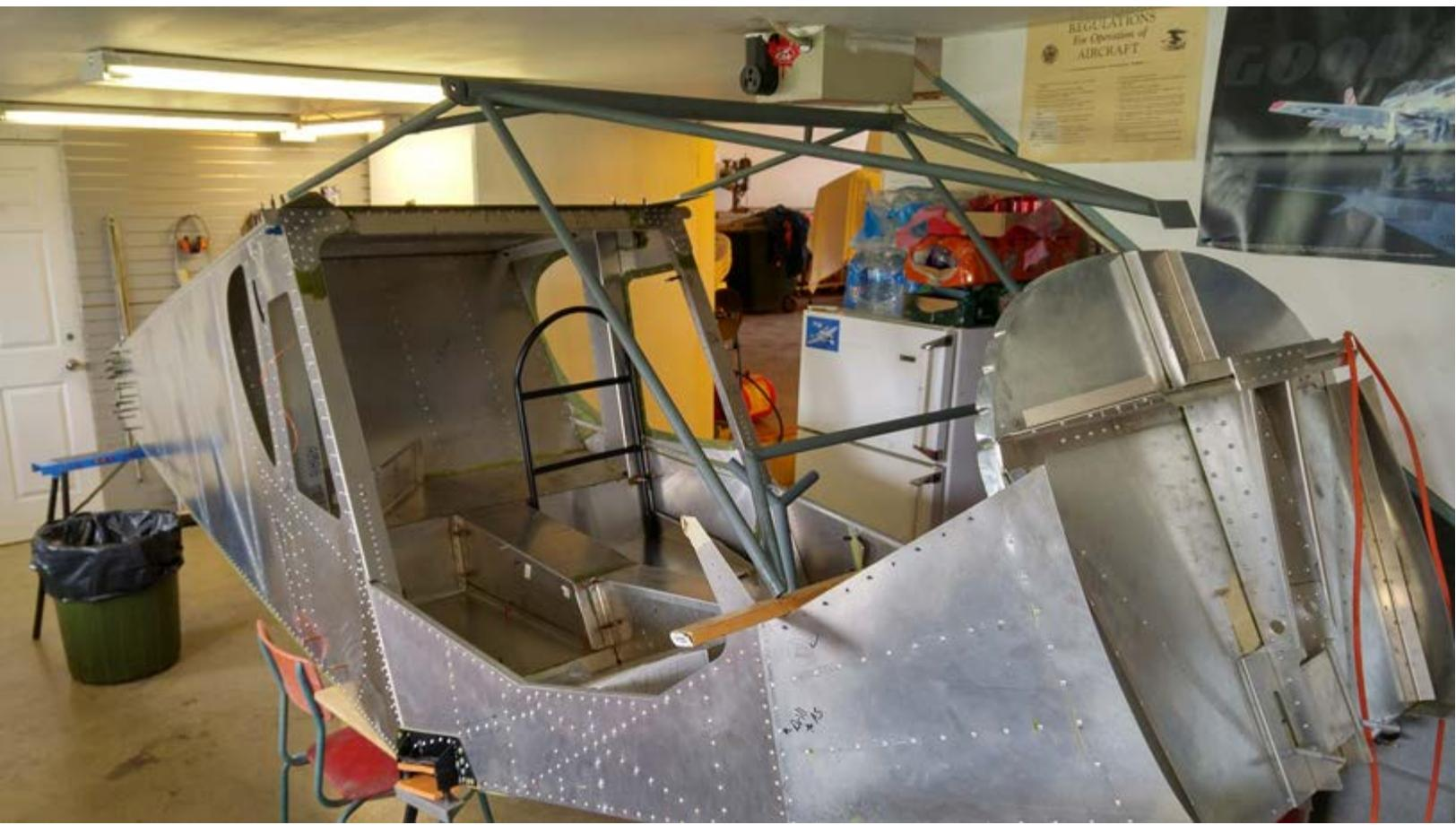
While work on the fuel lines was underway, another group was learning new skills by creating flared access holes in the baggage floor areas. It was decided to use nutplates for securing the access covers and we learned how to use a rivet squeezer to dimple the holes and then rivet on the nutplates with flush rivets. We also learned how to use a tool to install rivnuts to allow easy access to the area under the centre console, another enhancement we had decided on.
