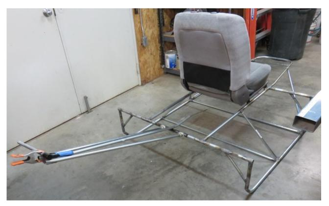
bottom and lateral loads are supported by a friction bearing made of a block of very hard wood. This block has four 5/16'' brass threaded inserts allowing it to be bolted to four 1/2'' EMT tubes welded to the seat platform
