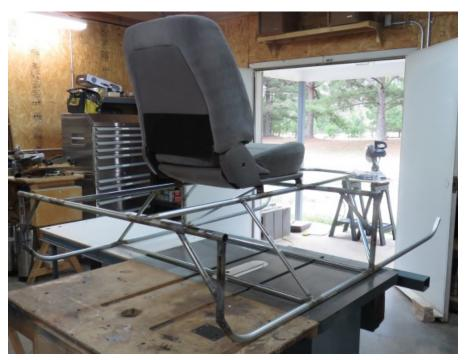
distance I bent  $\frac{1}{2}$ " EMT to form the peddle support frame and welded it in place. The picture below shows the results.
