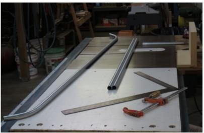
horizontal members to set the width of the frame. Then I cut the four vertical pieces (in two sets: two long and two short) which set the platform height on which the seat would sit.
