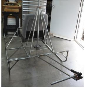
them at the rear end to form the beginning of the tail rotor system. This picture shows the beginnings of the tail boom along with the start of the tail rotor work.
