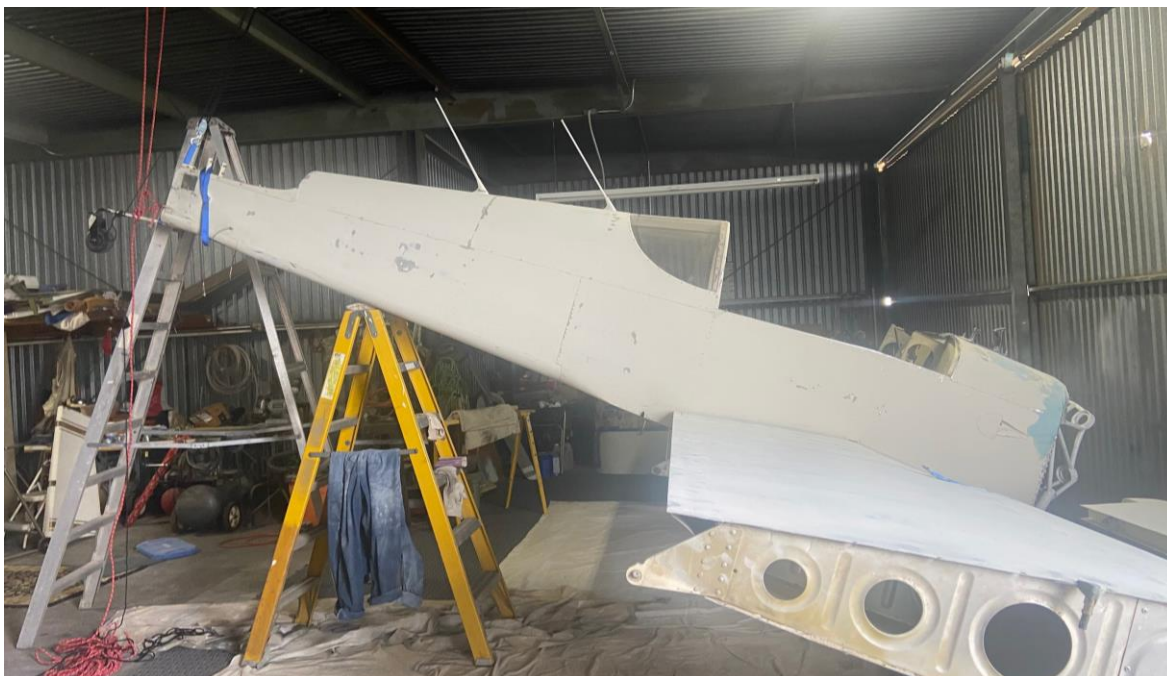
Tenley's RV-6 restoration project! How to wet sand the belly and bottom of the wing with sanding muck in your face! 🎉
