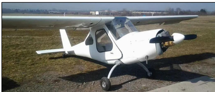
The fully Enclosed Ultralight Merlin with Front Cowling Off to Show Single Cylinder 2-cycle Polini Engine
