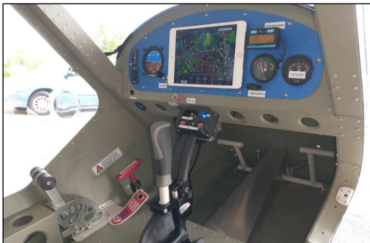
Merlin Available with Complete Instrument Panel and Ballistic Parachute, ready to fly. Note the Artificial Horizon Compass!
