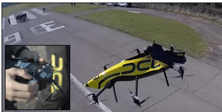
A Person on the Ground Controls the Manned Racing Drone.
