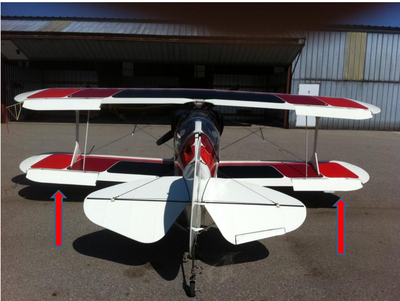
Position of ailerons upon engine shut down
