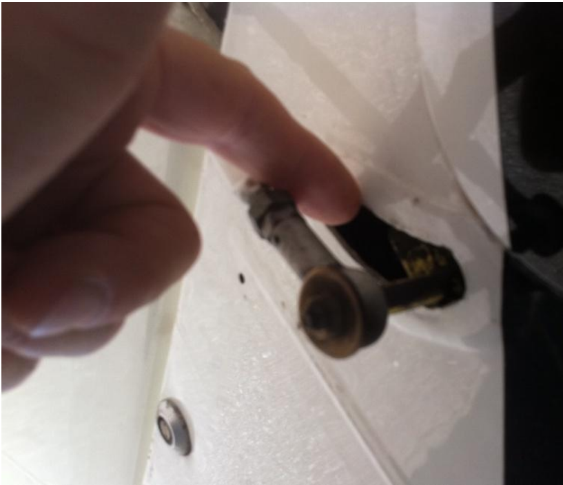
Slave rod assy loose and hanging down
