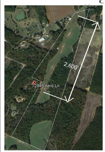
2,600' by 100' turf runway aligned 03 / 21 with additional 200' run off area,south end.
