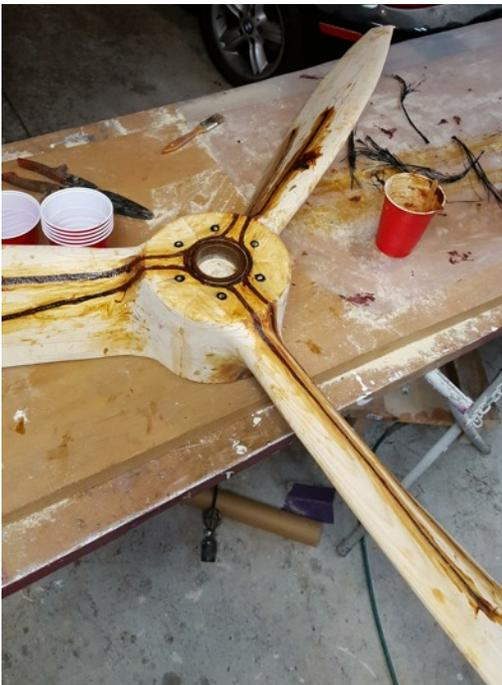
Fiberglass center hub with 1/4 diameter carbon fiber spars wrap around the hub and down each blade. So far very happy with the progress for the prop. It has taken 6 nights of carving to get this far.
