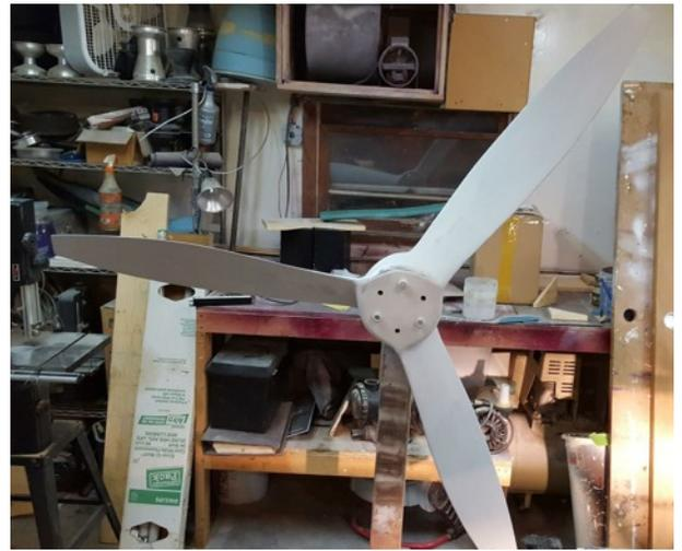
2 days after Flat side is glassed: Trailing edge of the prop wood is removed back about 3/8 of an inch before the shaped side of the prop is glassed. The glass is wrapped over the leading edge about 3/4 of an inch on the flat side of the blade. Once glass is stimped out, Peel Ply is added to control the glass from moving and to give a good surface to work with during the finishing process.
