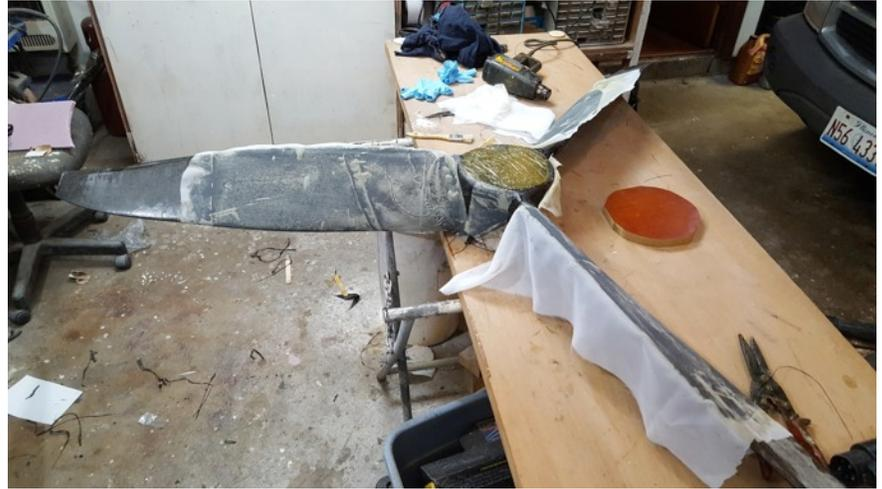
All bid is cut at a 45 degree angle. Uni all fibers run along the length of the blade.
