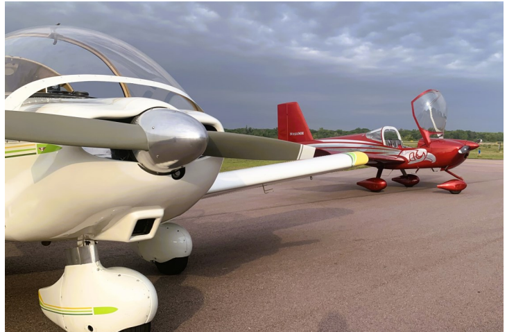
Zenith and Mike Howard's RV-12. The trim scheme on Mike's RV is interesting. The 'chrome' look is polished aluminum, with the metallic red paint over. Very nice!
