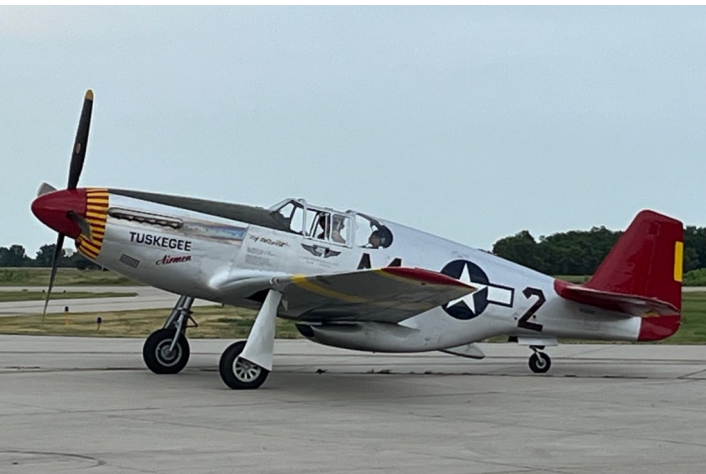
A real rarity - P51C Mustang in Tuskegee Airman markings. C models are a rare sight these days as most of them were left in situ or bulldozed after the war. The later D model offered better pilot visibility and other features learned for combat use.
