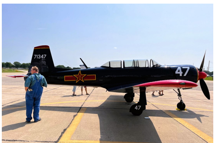
Nanching CJ6, Chinese Air Force trainer. Many of these have been imported into the US and provide warbird looks while being easier on the pocket book than a Mustang, Corsair or other exotic fighter. Fully aerobatic, the Nanching is quite popular.
