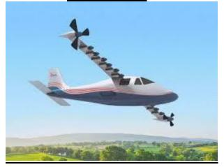
NASA's X-57 'Maxwell' is the agency's first allelectric experimental aircraft, or X-plane, and is NASA's first crewed X-plane in two decades. The primary goal of the X-57 project is to share the aircraft's electric-propulsion-focused design and airworthiness process with regulators, which will advance certification approaches for distributed electric propulsion in emerging electric aircraft markets.
