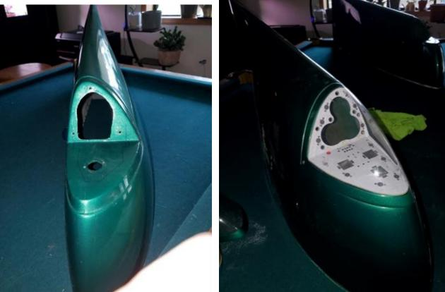
The PCB boards provided are slightly oversized and need to be trimmed to fit. I followed advice of prior kit builders and used my 3M scotch brite wheel on the bench grinder. Once done, I was able to test fit as shown in the next picture. Best to do this prior to soldering the components to the wingtip boards.
