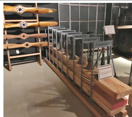
Ole's "Gluing Press" with stacks of 3/4" boards ready to become a single laminate, and then to become a carved propeller.
