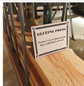
Ole's "Gluing Press" with stacks of 3/4" boards ready to become a single laminate, and then to become a carved propeller.
