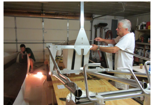
Here's the SeaRey fuselage and various metal components in the process of assembly in Dave's workshop garage at his home....very nice workmanship!
