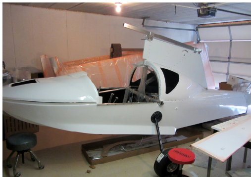
Here's the SeaRey fuselage and various metal components in the process of assembly in Dave's workshop garage at his home....very nice workmanship!
