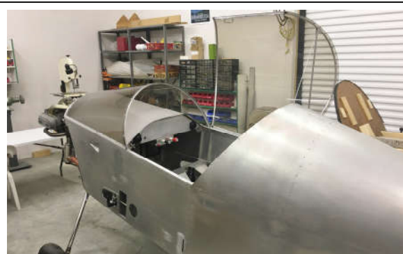
Canopy in “open” position. A cable holds the canopy from opening further, but I’ll likely need to make something to hold the canopy open in wind so it doesn’t come slamming down on sensitive body parts.
