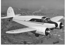
the Cessna T-50, Cessna's first twin-engine airplane) was nicknamed Bamboo Bomber by the pilots who flew them due to the use of spruce spars, spruce and plywood ribs, and plywood wing leading edges and wing tips. The fuselage is tubular steel and covered with fabric.
