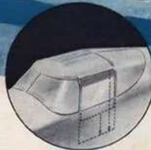
Arrows indicate how both top and side panels slide down into fuselage walls. A lock on top of side panels shuts against the inner cabin.
