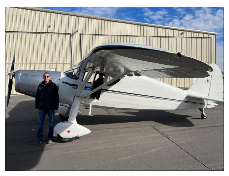
The F24 is a four-seat, single-engine, tailwheel aircraft designed by the Fairchild Aviation Corporation in the 1930s. It was adopted by the United States Army Air Corps as UC-61 and by the Royal Air Force. In terms of build, the F-24 embraces a retro-style, tough-as-a-tank mentality, with steel tubing running everywhere. She's ugly in a badass sort of way. Locker-room gossip has it that the load factors are north of 9 G's, although that's not something I
