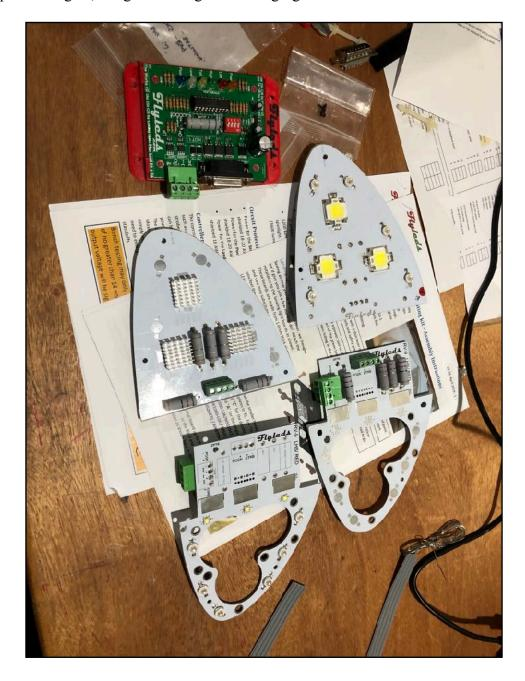
I ordered the kit from Flyboy Accessories, and it arrived a couple days later. Now, this is a kit, which means you get to practice your soldering skills. The kit consists of two circuit boards per wingtip, an integrated fully assembled combination tail strobe /position light, and a control board. The instructions are very complete with a bit of humor here and there, but you should read them over front to back before starting.
