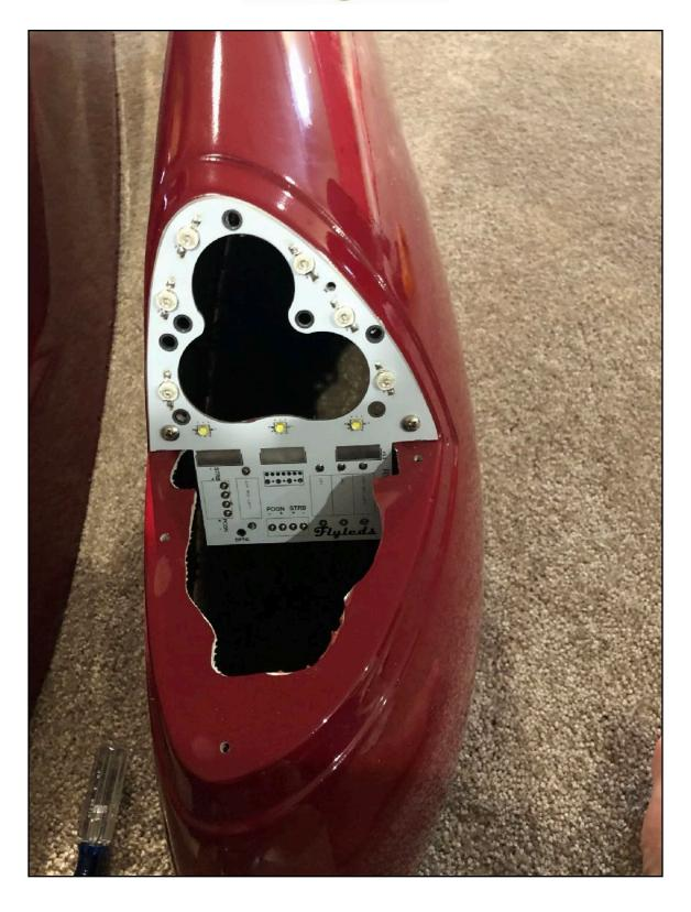
The wingtip installations went very quickly. The tail strobe took a couple attempts, as I initially cut the wrong wire leading back to the tail. Testing all the wiring on the bench using alligator clips is a very good idea.
