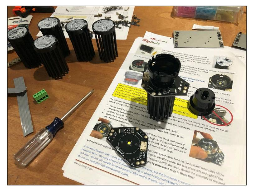
Margot & I pulled the fiberglass wingtips off the RV and brought them home. She removed the old lights while I started soldering up the control board. The soldering is fun, just take your time and make sure you put all of the components in the right places and facing the correct direction. A good soldering iron is a big help here.
