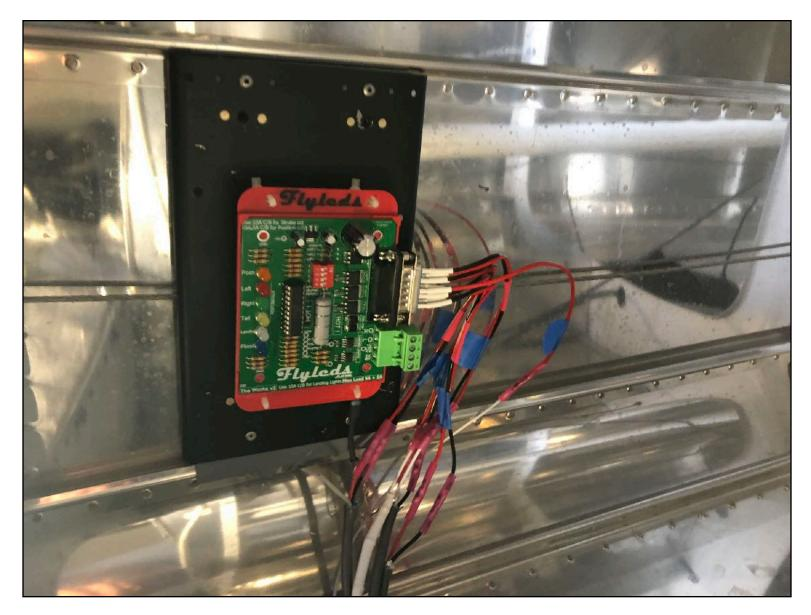
The control board mounted to the same plate that the old Whelen box was on. The kit even came with standoffs to mount it.
