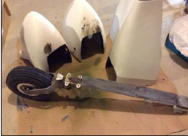
The second picture is of my repaired nose gear, ready for primer and paint. The wheel pants will also get some paint to cover the scrapes. I still have some work to do on the nose section of the plane but should be back in the air within a few weeks.
