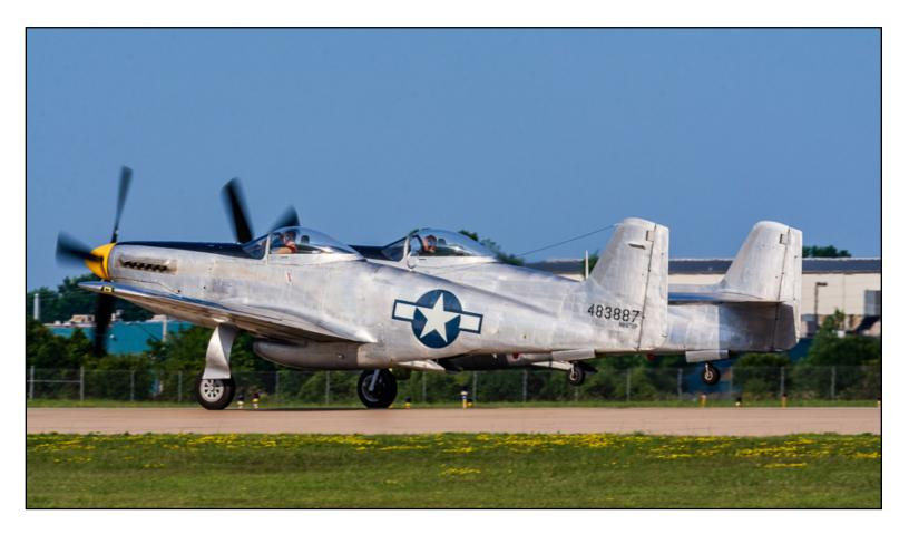
I will relate a couple details though, this airframe, the second prototype was first to actually fly in 1945, the design was intended for use as a long range escort for B-29 Super Fortress bombers in the Pacific. Its interesting to note that there are less than a half dozen components on the aircraft's airframe that are common with the P-51.
