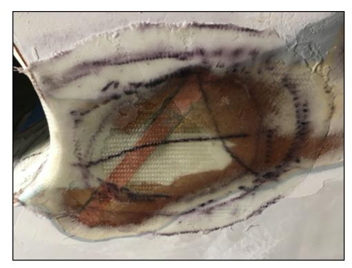
After the layup cured I sanded the rough edges and made up another batch of micro that I smoothed over the entire area. When that cured I sanded it down, ready for primer and paint:
