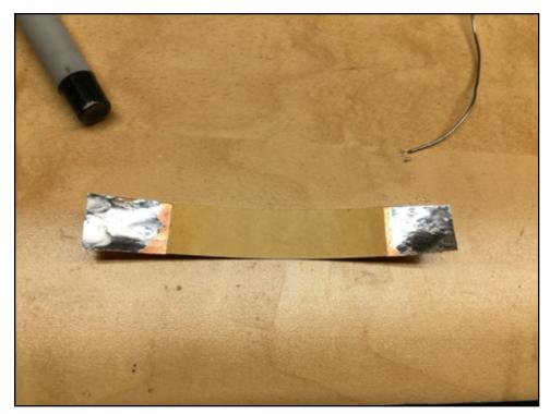
After filling in the damaged area, I very carefully cut away the fiberglass over the antenna to expose some of the copper foil on both sides of the damaged area. This was tedious as there were 3 layers of fiberglass cloth over the copper. After a while I was able to get sufficient copper exposed to make the repair. I cut a piece of copper foil long enough to join the two pieces and then tinned the ends:
