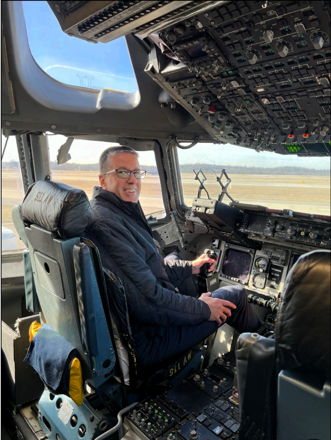
Danny Michaels in the cockpit of the C-17. Notice the stick control (no yoke).
