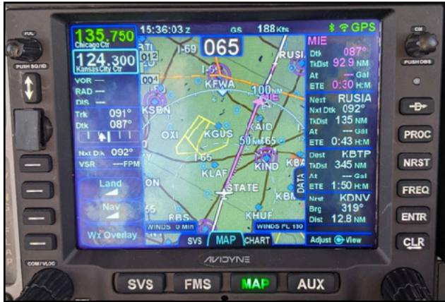
The IFD-550 has a heading input, making the wind correction angle obvious.
