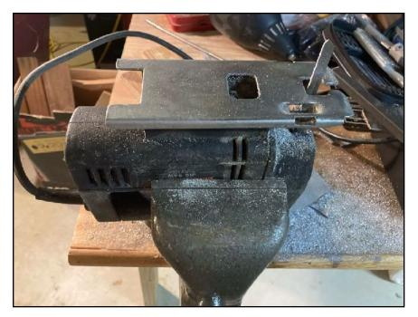
The best blade was a DeWalt bi-metal blade mounted with the teeth facing rearward, as you can see in the photo. With some elbow grease and cutting oil I got the cuts made. A second cut had to be made that the jigsaw could not make, so I used a diamond coated cutoff wheel in my Dremel:
