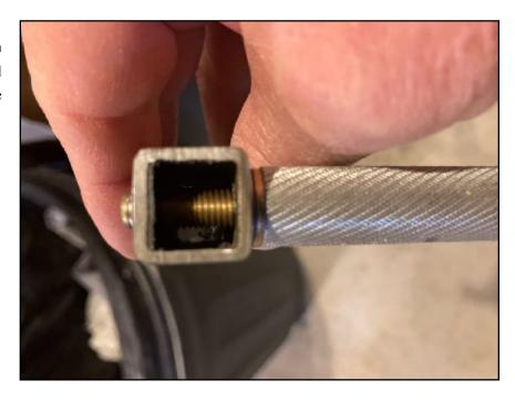
After some filing and grinding to remove any rough edges I cleaned the parts with an abrasive brush in a drill:
