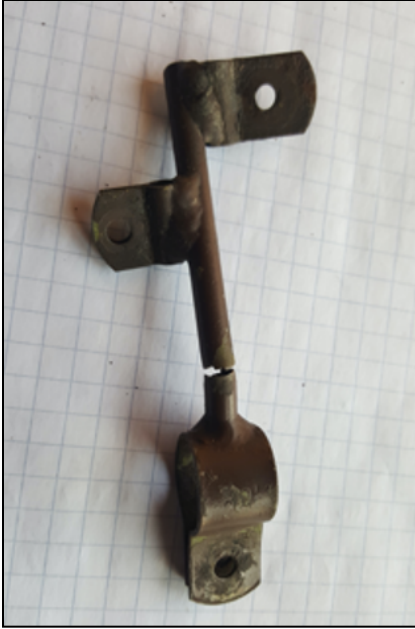
Fig 3. Throttle and mixture cable bracket assembly removed from light single engine airplane. The bracket tube has broken and separated near a clamp at the bottom of this photo, which attaches to the engine mount.
