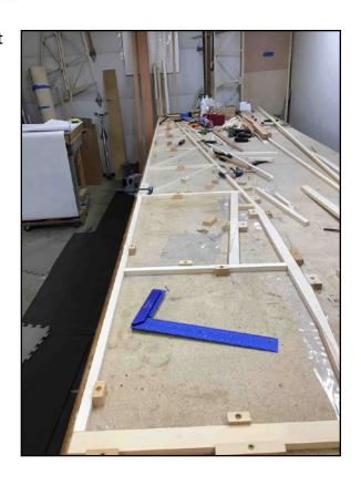
Fuse side2 is a shot of the 2nd fuselage built on top of the 1st side.
