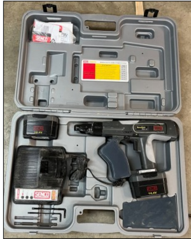
Senco Drywall Screw Gun, needs new battery(ies) which can be found online for around $40
