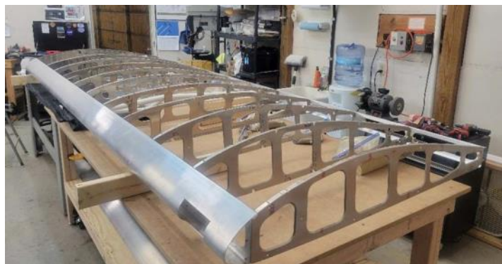
Left wing structure.
