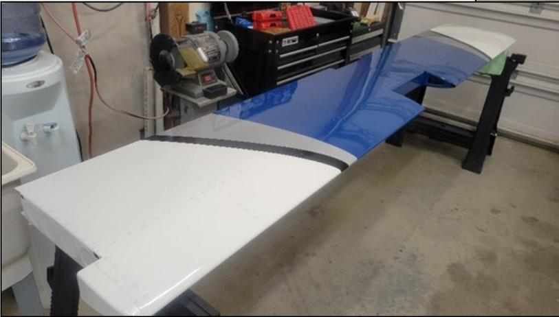
The paint is pretty easy to spray once you get the technique. I've had to scuff sand and re-do a couple things due to orange peel which has slowed down the process.
