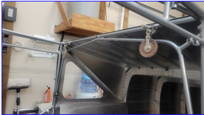
Aileron Cable Pulleys
