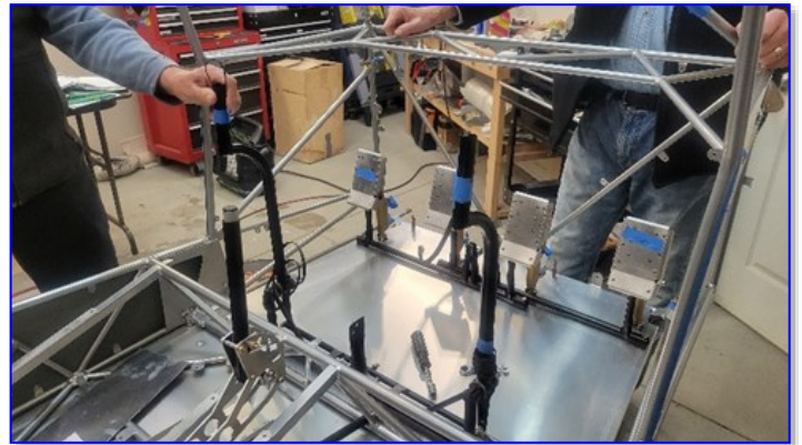
Rudder Pedal and Control Stick Assembly Install
