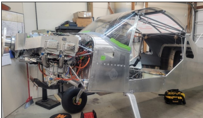
Windshield and Skylight finally installed after countless fittings.
