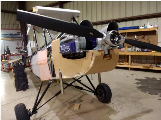
The new cowl is designed to show off Azalea's Corvair Aero-engine conversion to good effect and promises to be a head turner with new graphics and colors added.
