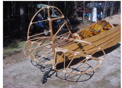
The fuel shut off and elevator trim controls were fabricated, and the cables were fitted and installed. I put the rudder, horizontal stabilizer, and elevator temporarily to check fit and to get the proper length for the elevator trim cable. Several brackets for the upper wing mount tubes have been fabricated. The lower wings and ailerons are mostly complete.
