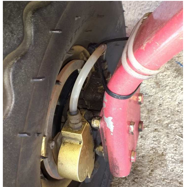
Big air in brake line. The dual puck brakes should have the crossover underneath to allow full bleeding. Note the black zip-tie holding the cross-over from dragging on the tire....
