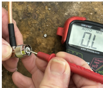
Gripping insulated handle w/o touching metal probe results in no short circuit indication.
